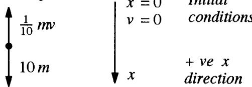
$$m\ddot{x} = 10m - \frac{1}{10}mv \quad \therefore \ddot{x} = 10 - \frac{1}{10}v$$
